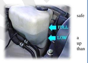
Some vehicles' recovery tanks are pressurized when the engine is hot, making the caps as dangerous to remove as radiator caps. Pressurized recovery tanks are clearly marked with warning decals and their cap is a system pressure cap, rather than a simple plug or twist-off cap.
